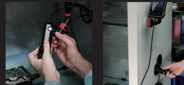
The small camera-head can be put into a device such as thermostatic chambers. You can operate remotely by touchscreen of the external controller while checking the measurement status.
