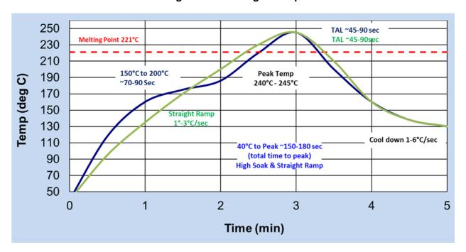
Figure 1 – OM-358 SAC305 & Innolot General Reflow Profile Recommendation
