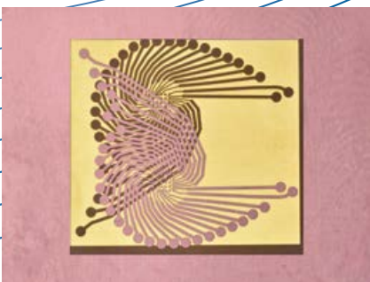
Removal of copper from double-sided PET film
