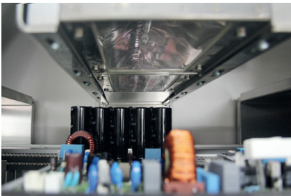
High-performance lamps in the RDS 1200 UV for drying all UV-hardened coatings
