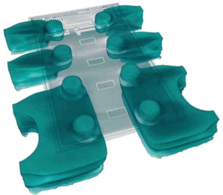
3D-CT volume of a microchip with pillar array
